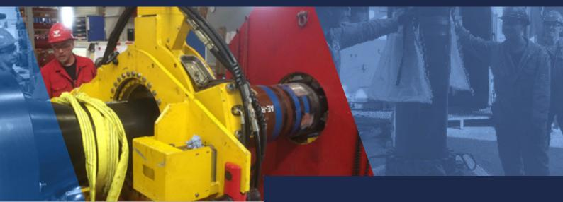
The Aquaterra Energy supplied VAM-TTR HP subsea high-pressure drilling riser is a 14" Nom Bore with VAM-TTR threaded and coupled pin and box connections, allowing for fast and efficient rig make up. The system was developed in response to strong market demand for a gas tight 14" bore subsea riser.
