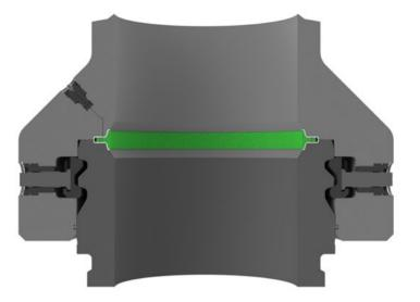
Preloaded static connection designed and qualified for dynamic loading
