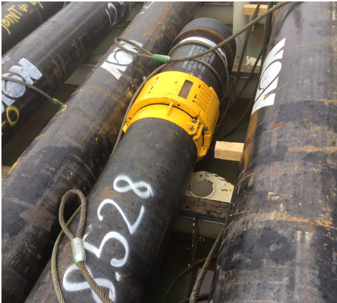
Pre-installed through rotary table slim line SUREGrip (for none starter head applications)
